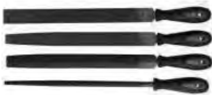
Hand files Used to abrade the edges of the sheet metal until smooth
