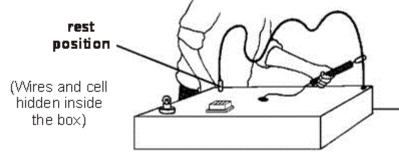
The metal ring and the thick wire both let electricity through.
